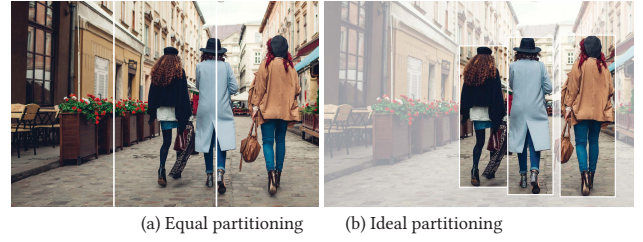
Figure 1: Examples of video frame partitioning. The simple partitioning method in (a) split pixels of the same object into multiple parts and yield poor inference results. We can achieve much better partitioning using ELF, close to the ideal partitioning shown in (b)
